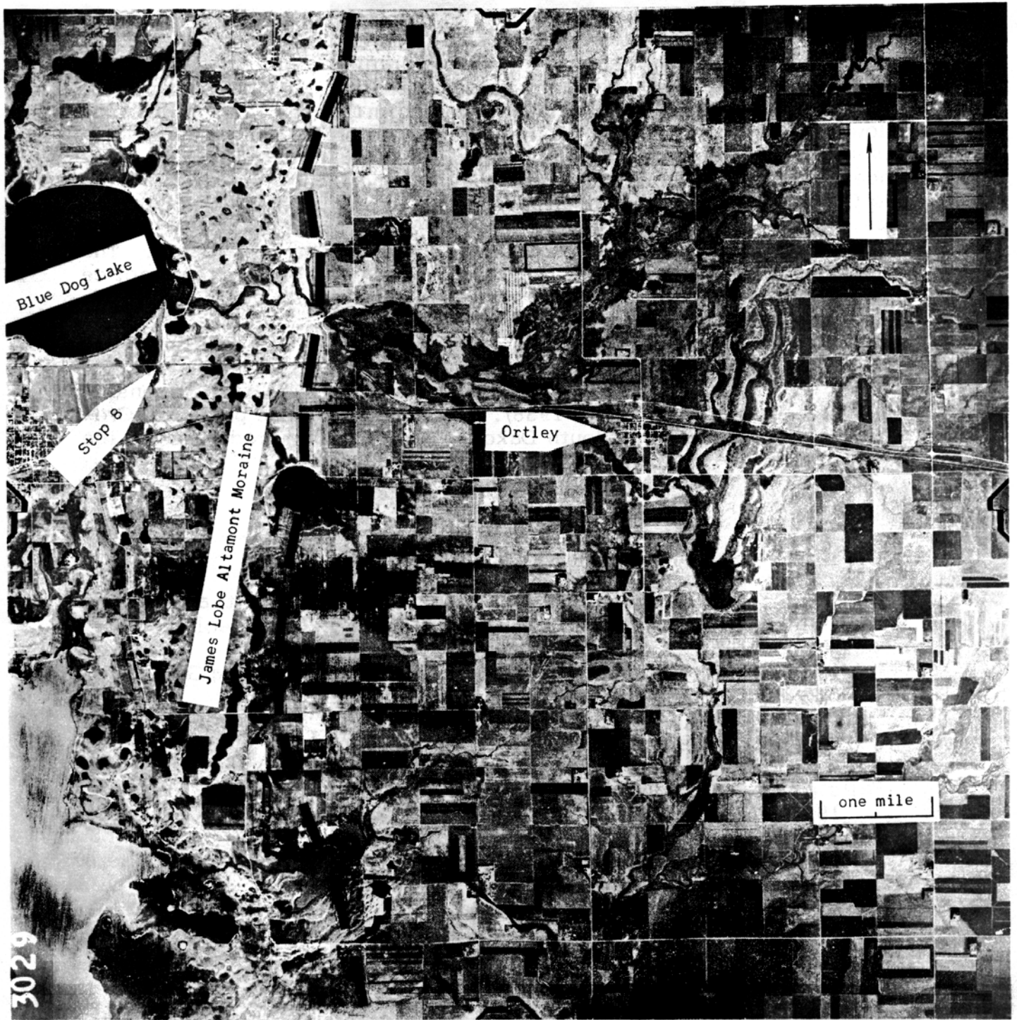
Figure 5-2. Vertical air photo of Blue Dog Lake - Ortley, South Dakota area, of Stop 5-3, showing James Lobe Altamont moraine as compared with Des Moines Lobe Altamont and Bemis shown on figure 5-1. Location shown on figure 4-1.
