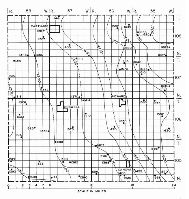
Well. Number is altitude of water level above National Geodetic Vertical Datum of 1929.
