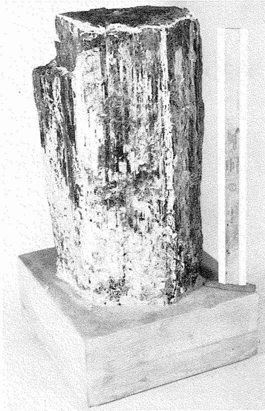
19A. Large schorl crystal showing hexagonal prism and basal hemipinacoid. The scale is one foot in length. Ross Lode.
