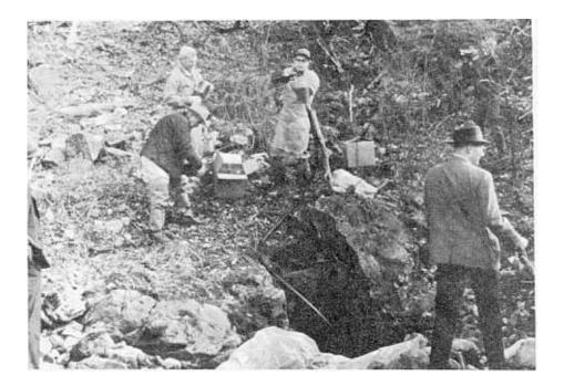
Figure 8. Dumping dye into the sinkhole in the Pahasapa Limestone along Boxelder Creek.
