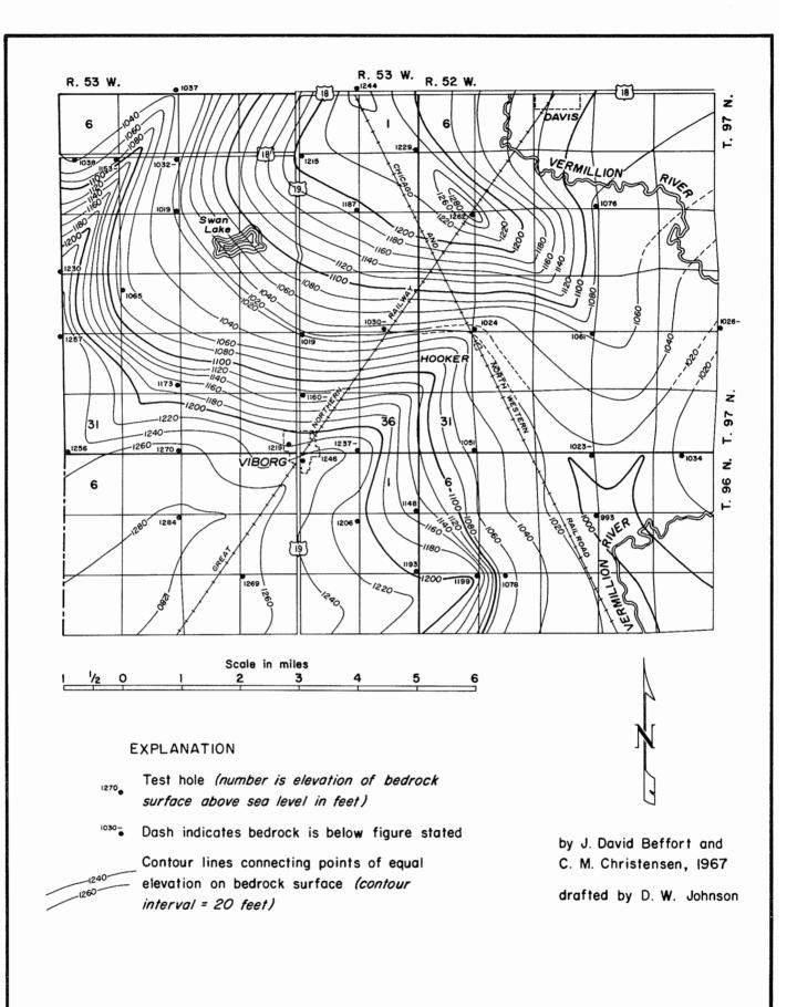
Figure 3. Map showing configuration of the buried bedrock surface in the Viborg area.
