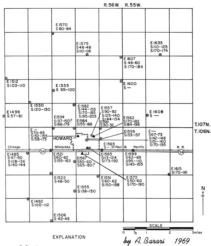
E = Elevation S IIO-I25 = Sand from depth of IIO to I25feet. Test hole drilled by S. D. G. S. Rotary rig
