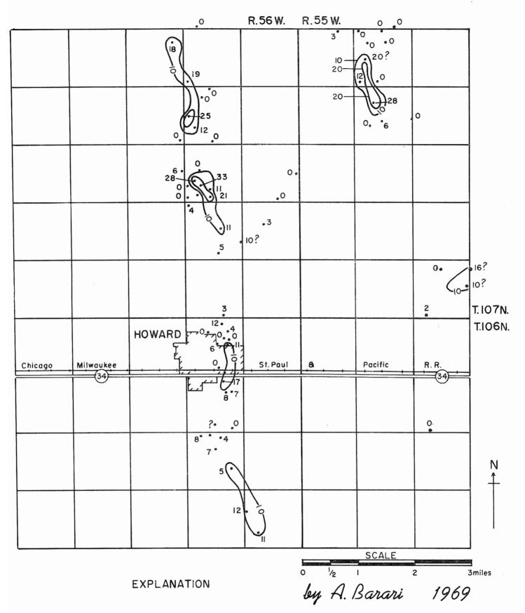
•12 Test hole showing thickness of saturated sand and gravel.
