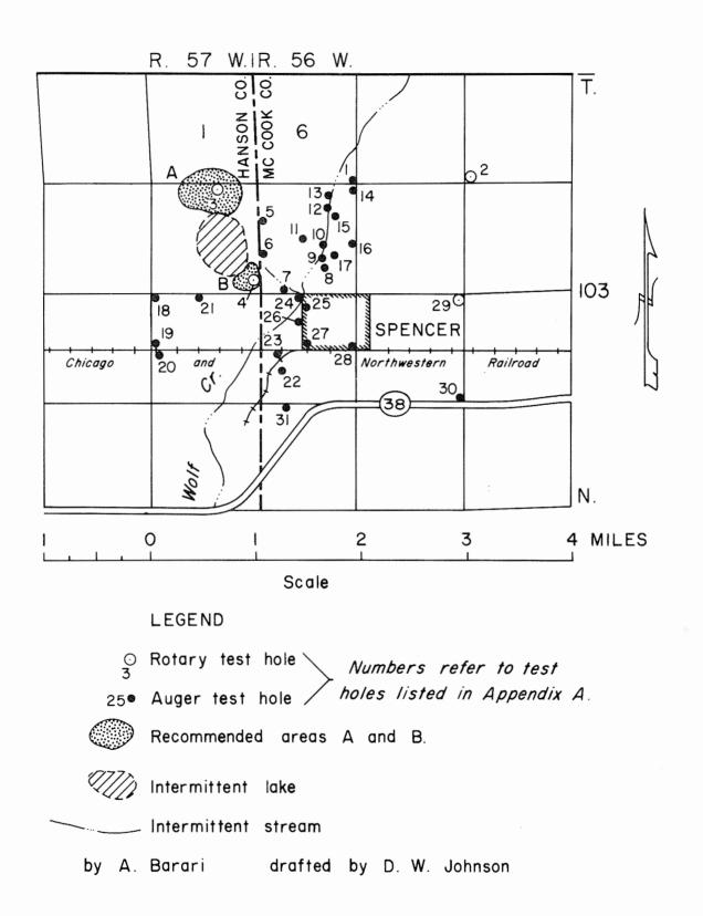
Figure 3. Map showing location of rotary and auger test holes in the Spencer area.
