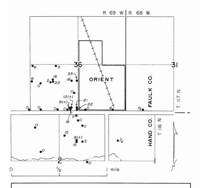
Test holes located in the Orient area-numbers refer to total thickness of sand and/or gravel. A plus (+) indicates the total thickness of sand and/or gravel was not penetrated. (for test hole number and depth to sand see Figure 3 and Appendix A.)
