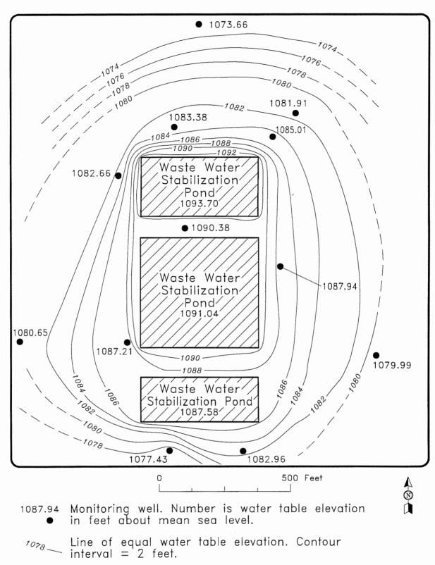
Figure 3. Water table elevations on September 30, 1992.
