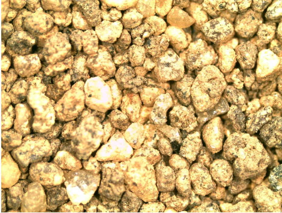
Figure B-3. Sample 2; magnified coarse sand; #35 sieve.
