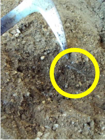
Figure 15. White scratch at sample location 2.
