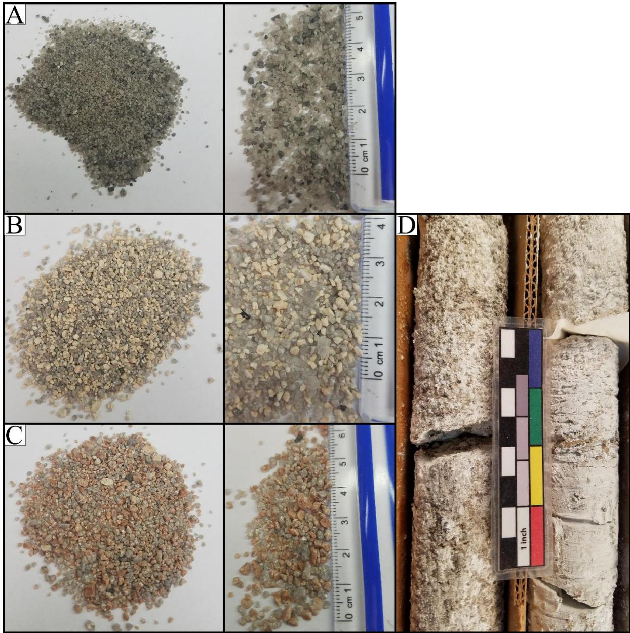
Mud-rotary cuttings from the granite wash aquifer (A) and the Milbank Granite regolith (B & C). The sand of the granite wash aquifer is void of feldspars (A).
